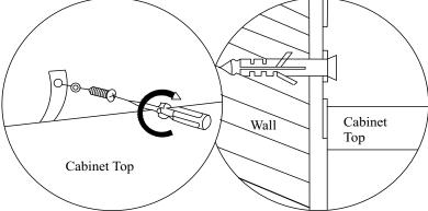
NOTE: Wall Fixings are not supplied with this product as different wall materials require different types of fixing devices (such as Rawl plugs on brick work) You must use fixing devices suitable for the type of wall you intend to mount this product to. Please ensure that the head of any screw used has a diameter greater than the diameter of the mounting hole on the product and that the fixing is safe and secure before use.
